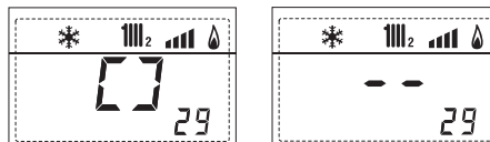
30. Solar sensor temperature with solar board
